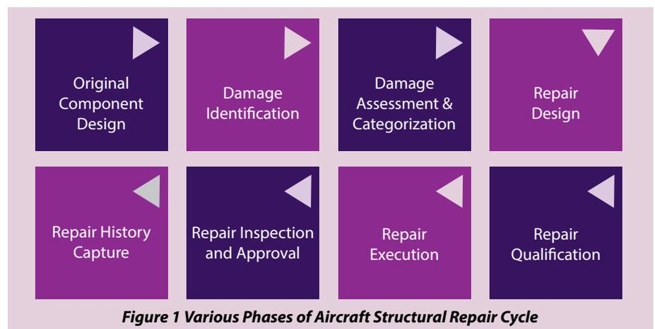
**Figure 1 Various Phases of Aircraft Structural Repair Cycle**
