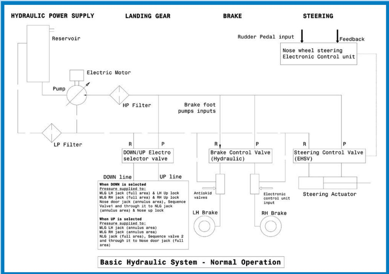
Fig. 3 Basic Hydraulics System – Normal Operation
