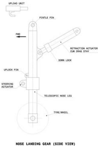
Fig. 1 Nose Landing Gear - Side View
