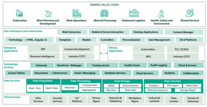
This digital architecture could help mining companies be agile and digital at scale, and generate roadmaps and solutions for future-readiness. It could help them collect real-time data from smart sensors, as well as, access data from legacy PLC, SCADA, MES systems and make it available in on-premises data warehouses on **Digital Architecture for Mining**
