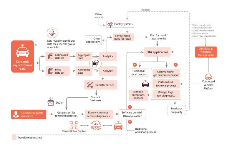
Remote diagnostics is an exciting area ripe for transformation wherein the need for the physical presence of a car in the workshop is eliminated, and instead the diagnostic information is sent to the workshop using connectivity. This brings up an entirely new aftermarket model.
