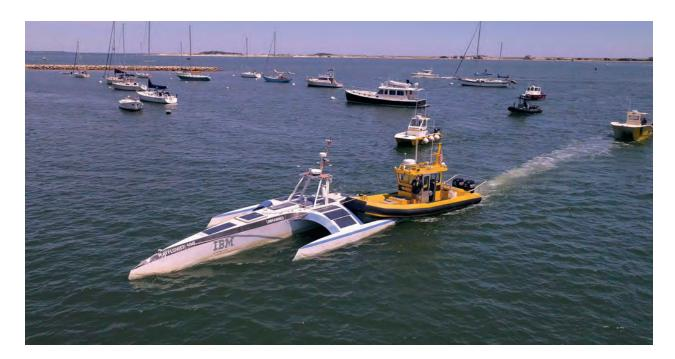
Edge computing is being used on the oceans, and even in space. The Mayflower autonomous ship (pictured above), a marine research vessel, gathers data about the ocean and makes its own Al-powered decisions about its route, status and mission, thanks to 15 edge devices that allow the ship to operate independently. It syncs with the cloud and uploads data and downloads updates when it gets a connection.
