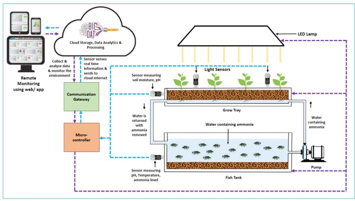
Figure 4 Schematic Diagram of Implementation of IoT in Vertical Farming
