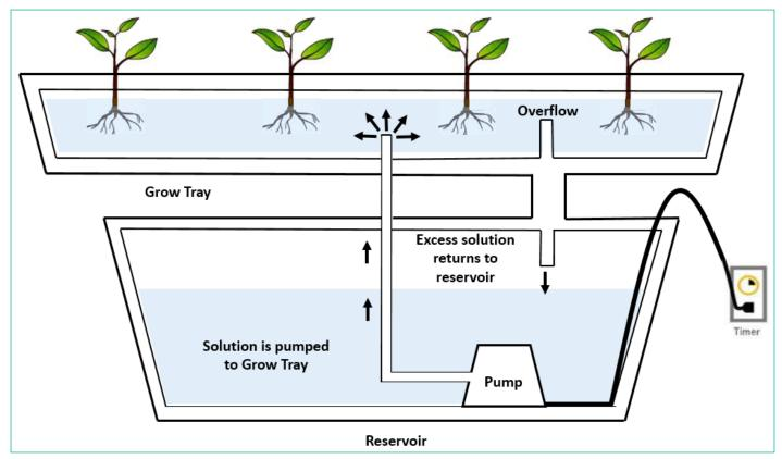
Figure 1 Schematic diagram of a hydroponic system
