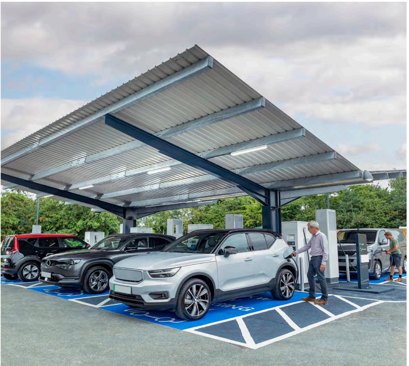
designing ADA-compliant charging stations, it is essential to consider accessibility, ease of use, and safety for disabled drivers, including those using wheelchairs or other assistive equipment. Key considerations include adequate space for entering and exiting of vehicles, unobstructed access to charging stations, free movement around charging stations, clear connection points on vehicles, and clear paths and proximity to any building entrances.
