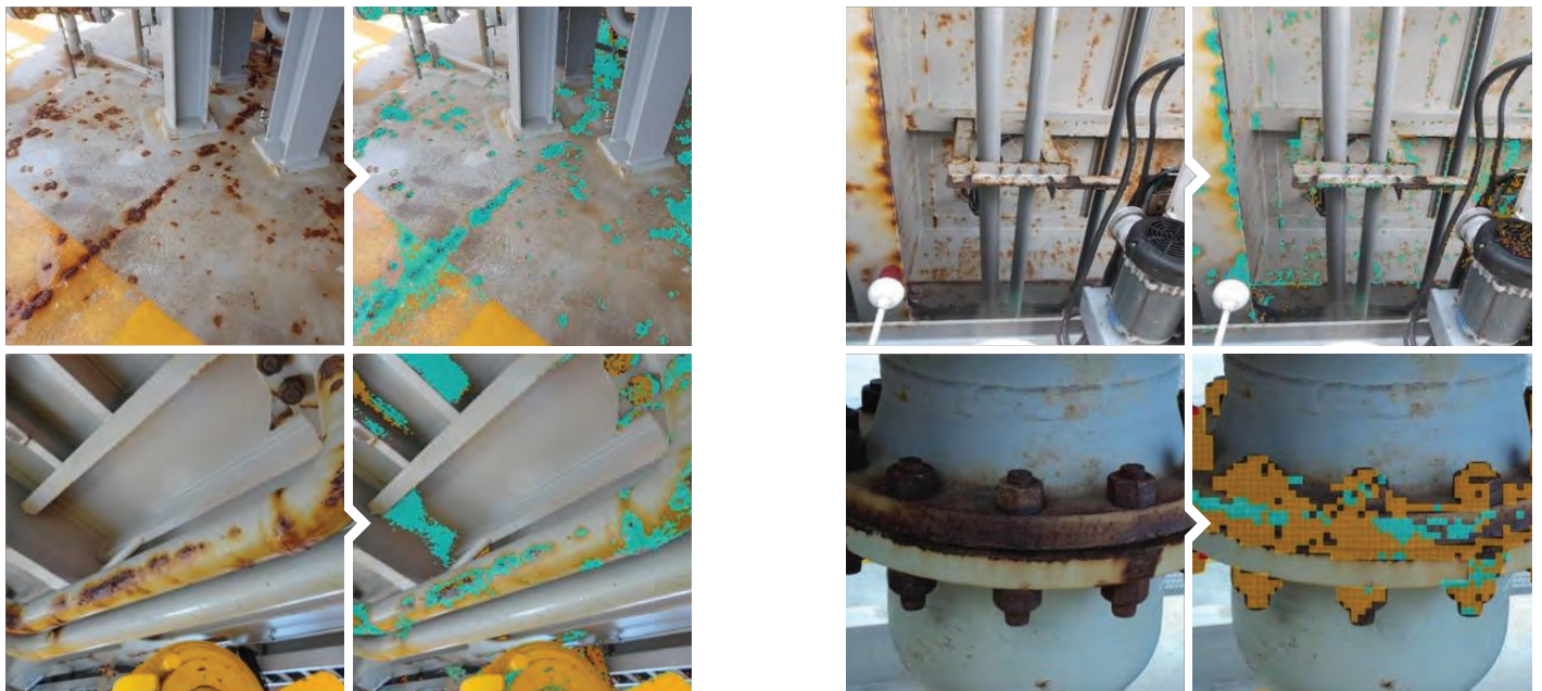
Figure 6. How computer vision sees corrosion
