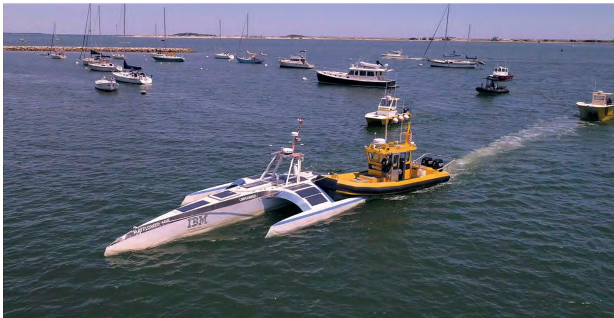
Edge computing is being used on the oceans, and even in space. The Mayflower autonomous ship (pictured above),<sup>6</sup> a marine research vessel, gathers data about the ocean and makes its own AI-powered decisions about its route, status and mission, thanks to 15 edge devices that allow the ship to operate independently. It syncs with the cloud and uploads data and downloads updates when it gets a connection.
