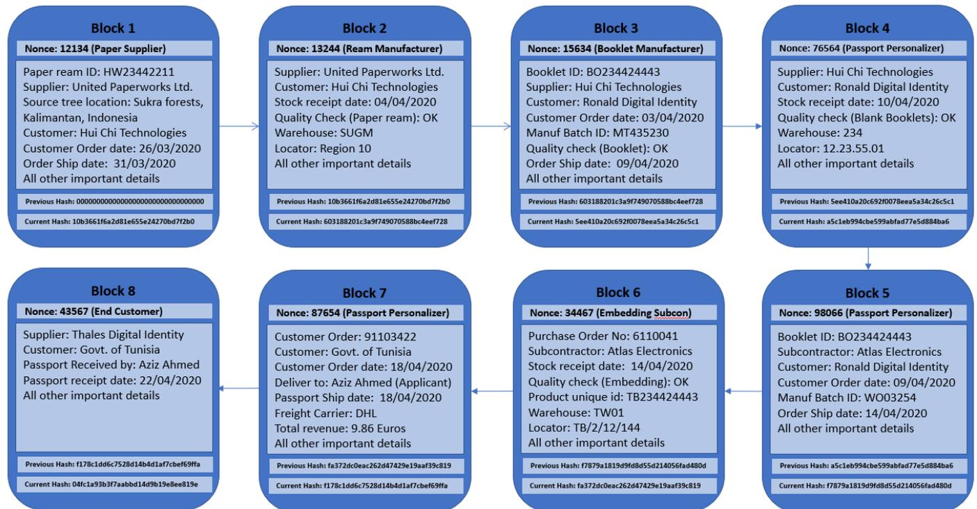
Figure 2: Blockchain representation of a passport supply chain
