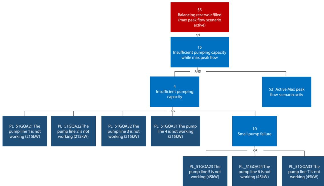
Fig 2: RAMS model for a pumping station
