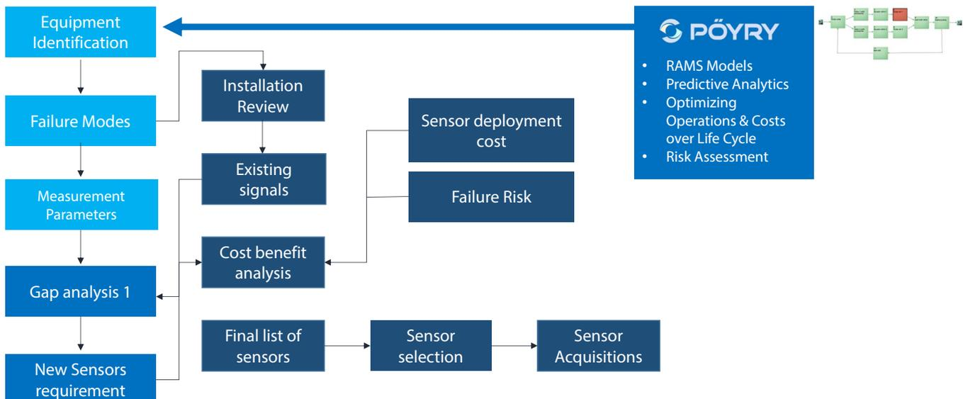
Fig 3: Workflow for sensor identification
