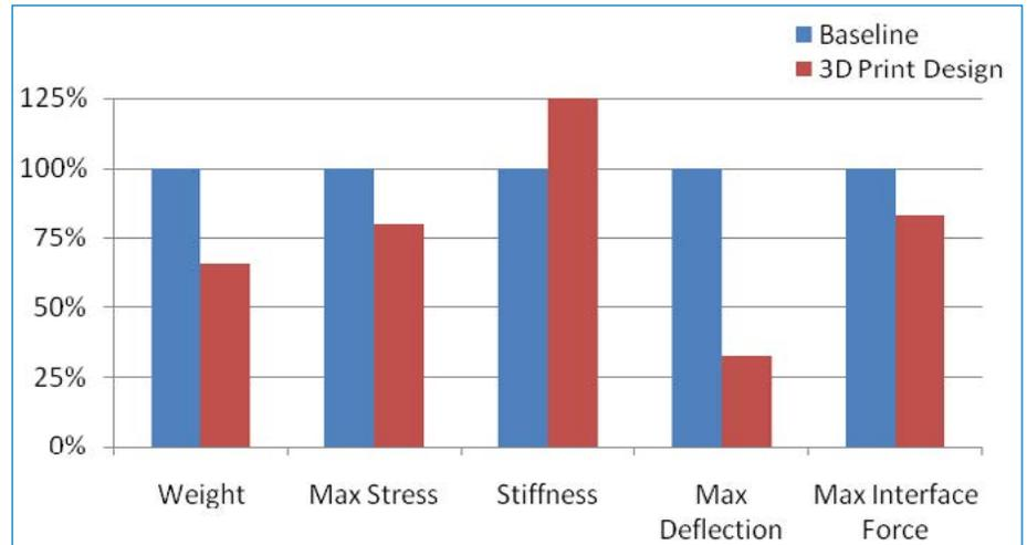
Figure 12: Comparison between current and optimized design
