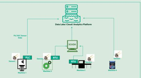
Automated Machines such as PLC Machines have sensor data that are stored within the machine. SCADA systems use Remote Terminal Units (RTUs) to get data from machine sensors in its ecosystem. Complete Shop Floor Visibility will be obtained when all the different machine data are connected and analyzed for better control, pattern detection and downtime minimization
