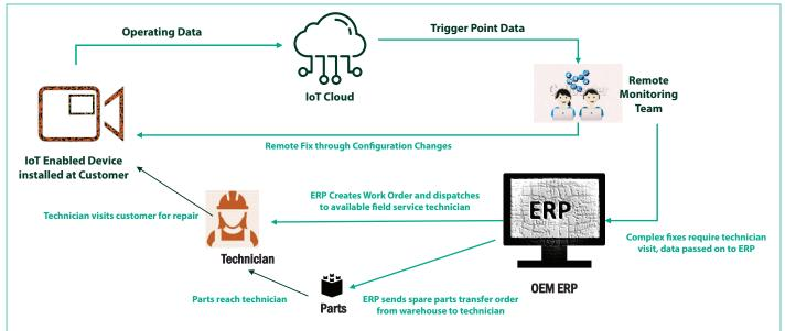
IoT enabled Devices reduce service costs by sending operating data, which allows certain fixes to be done remotely, thereby reducing field technician visits
