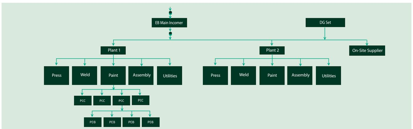
Figure 4: Sample Electrical Distribution Line Diagram
