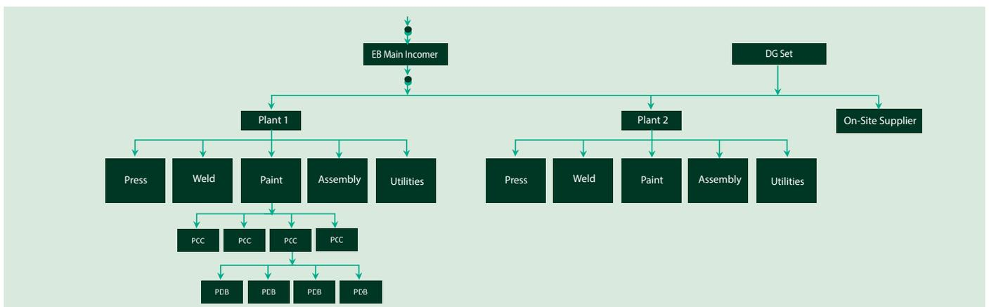
Figure 4: Sample Electrical Distribution Line Diagram
