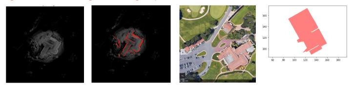
Fig. 23 (c): ML on RGB and thermal images for 3-D building reconstruction and thermal anomaly detection<sup>125</sup>
