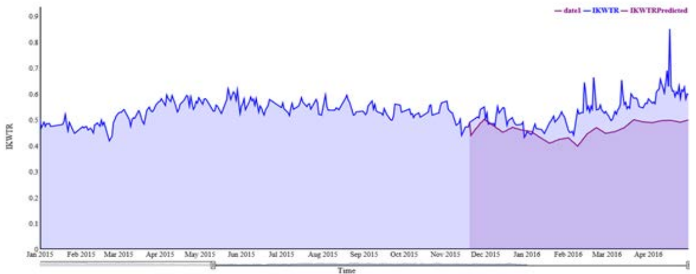
Figure 12: IKWTR forecasting using ARIMA with xreg = wet bulb temperature for GEC1_Chiller1
