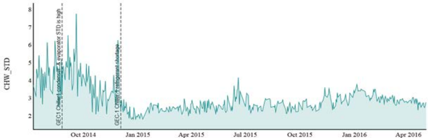
Figure 3: Chilled water, small temperature difference (CHW_STD) variation and maintenance events for GEC1_Chiller 1
