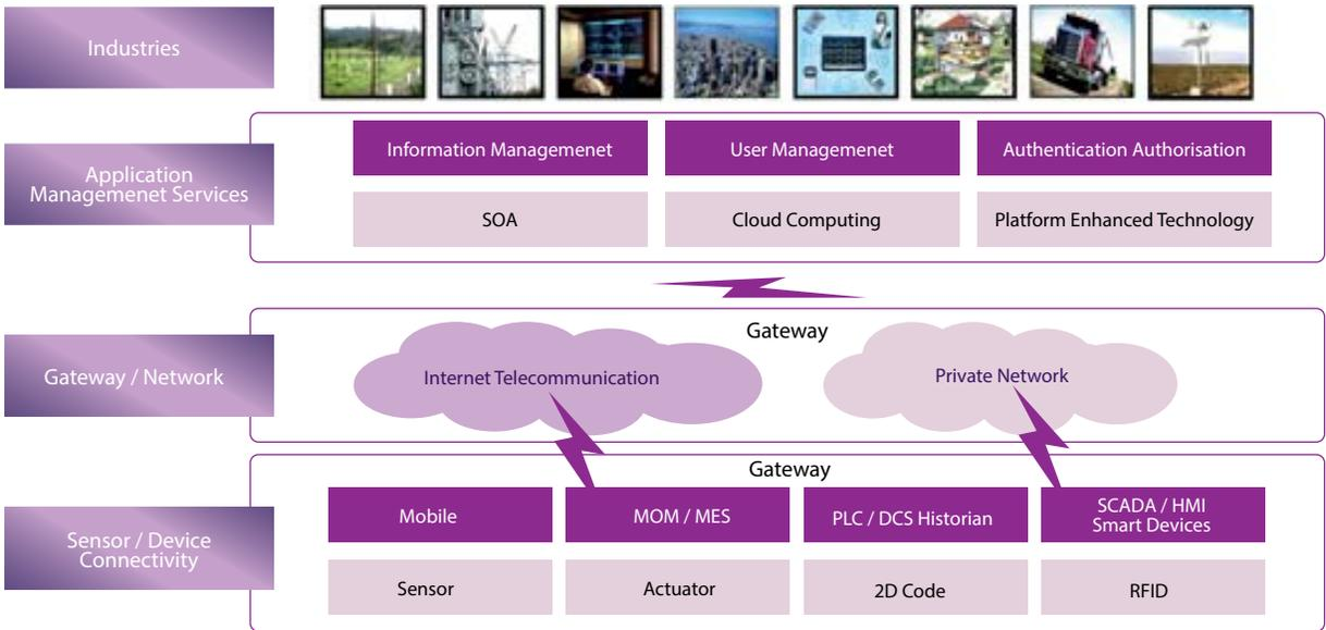
Figure 4: Layered IoT-based architecture for track and trace technologies
