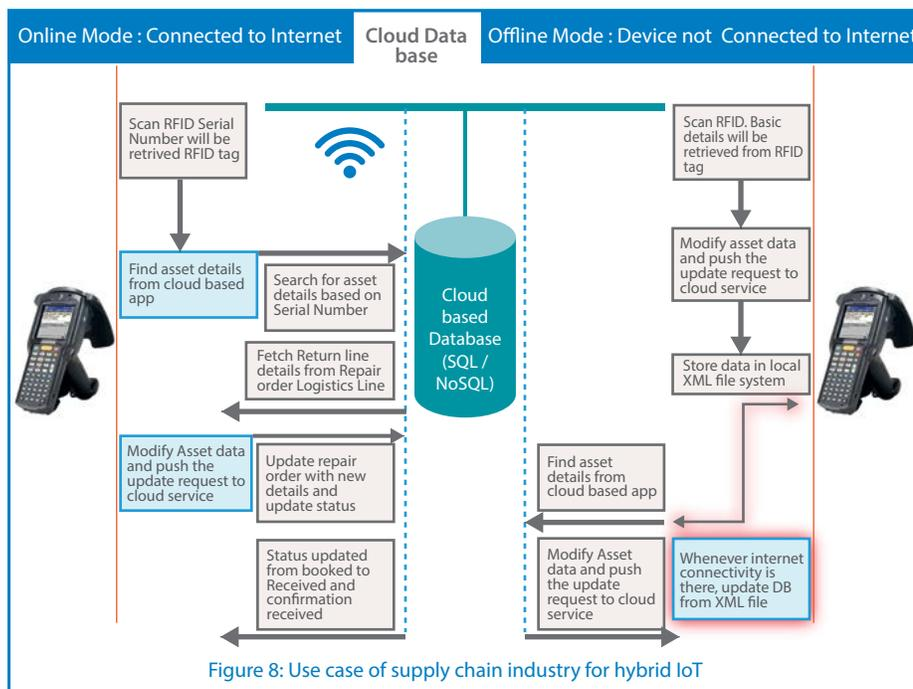
Figure 8: Use case of supply chain industry for hybrid IoT
