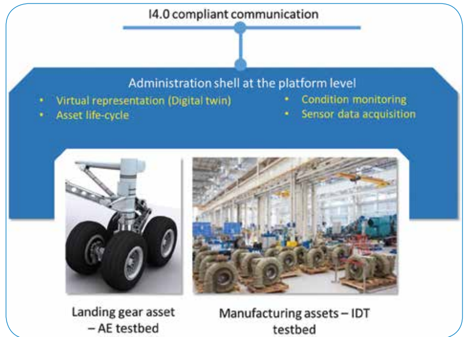
Figure 7 : I4.0-compliant landing gear (AE testbed) and products manufactured on a factory floor (IDT testbed) showing the administration shell that resides in the platform tier.
