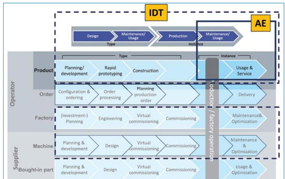
**Figure 6 : Various I4.0 components as detailed in the RAMI 4.0 architecture document (Source: M. Hankel, Bosch Rexroth. Based on Plattform Industrie 4.0 WG3. Based on Prof. Bauernhansl, Fraunhofer IPA. Copyright “Umsetzungsstrategie Industrie 4.0 – Ergebnisbericht, Berlin, April 2015”) showing the scope of the IDT and AE testbeds by means of the dashed and solid lines, respectively.**
