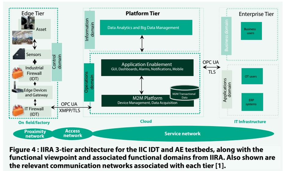
**Figure 4 : IIRA 3-tier architecture for the IIC IDT and AE testbeds, along with the functional viewpoint and associated functional domains from IIRA. Also shown are the relevant communication networks associated with each tier [1].**
