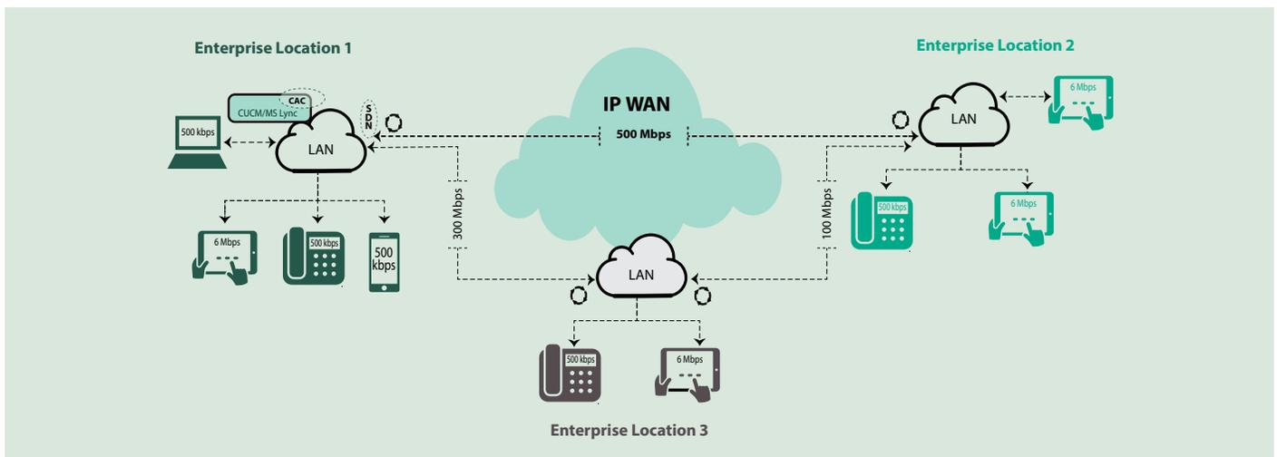
Figure 5. Dynamic Bandwidth Allocation in Enterprise Network
