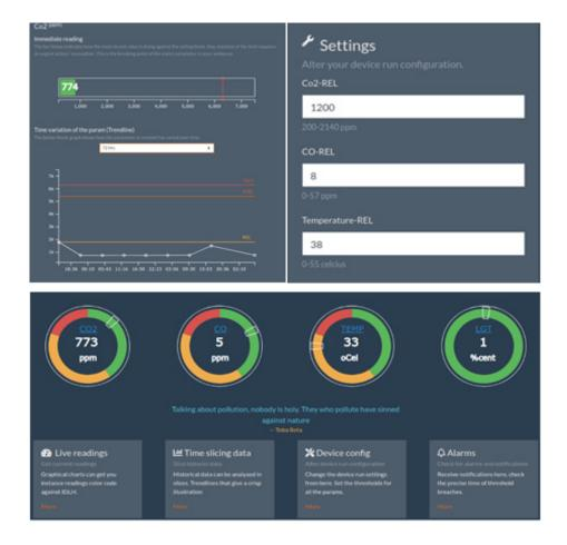
A Web application runs alongside the device always reading and analyzing current values of the confined space workplace. Graphic dashboards in the application display the trends and instance readings. The panel can be used to change the settings of the device and other sensor settings.
