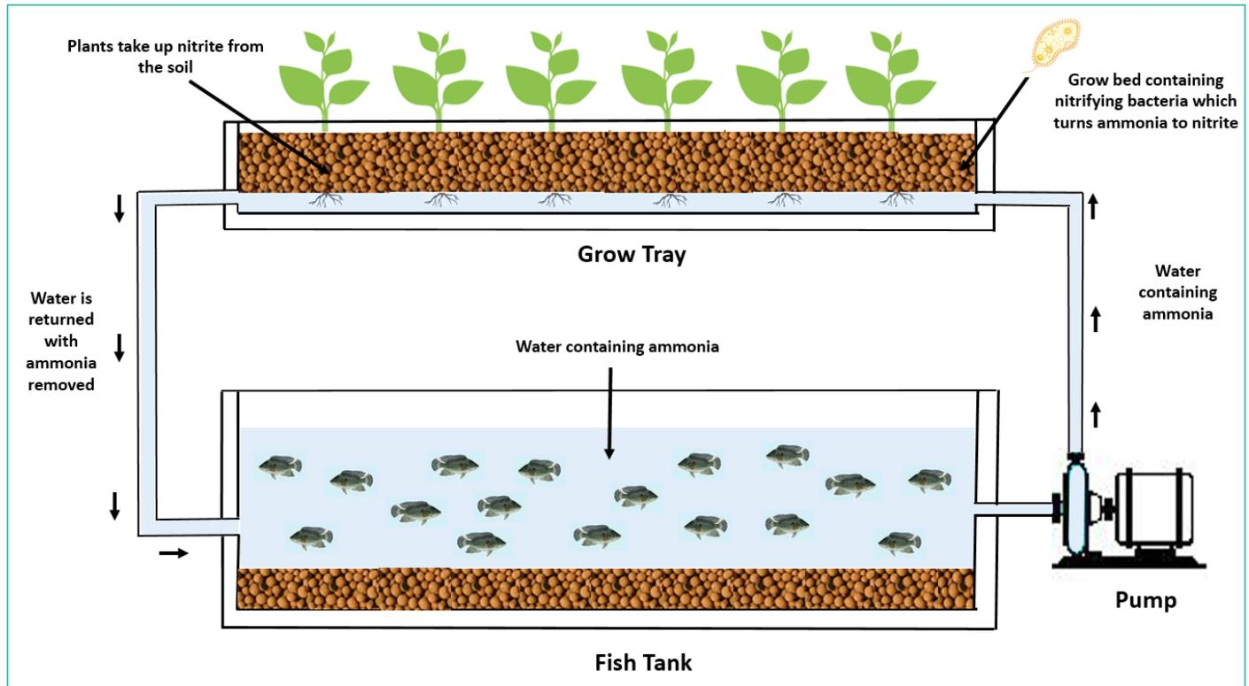
**Figure 3** Schematic diagram of an aquaponic system
