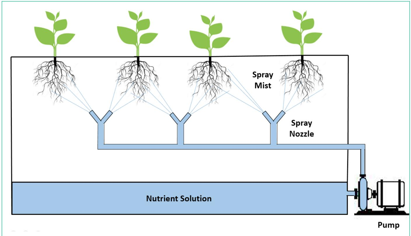
**Figure 2** Schematic diagram of an aeroponic system
