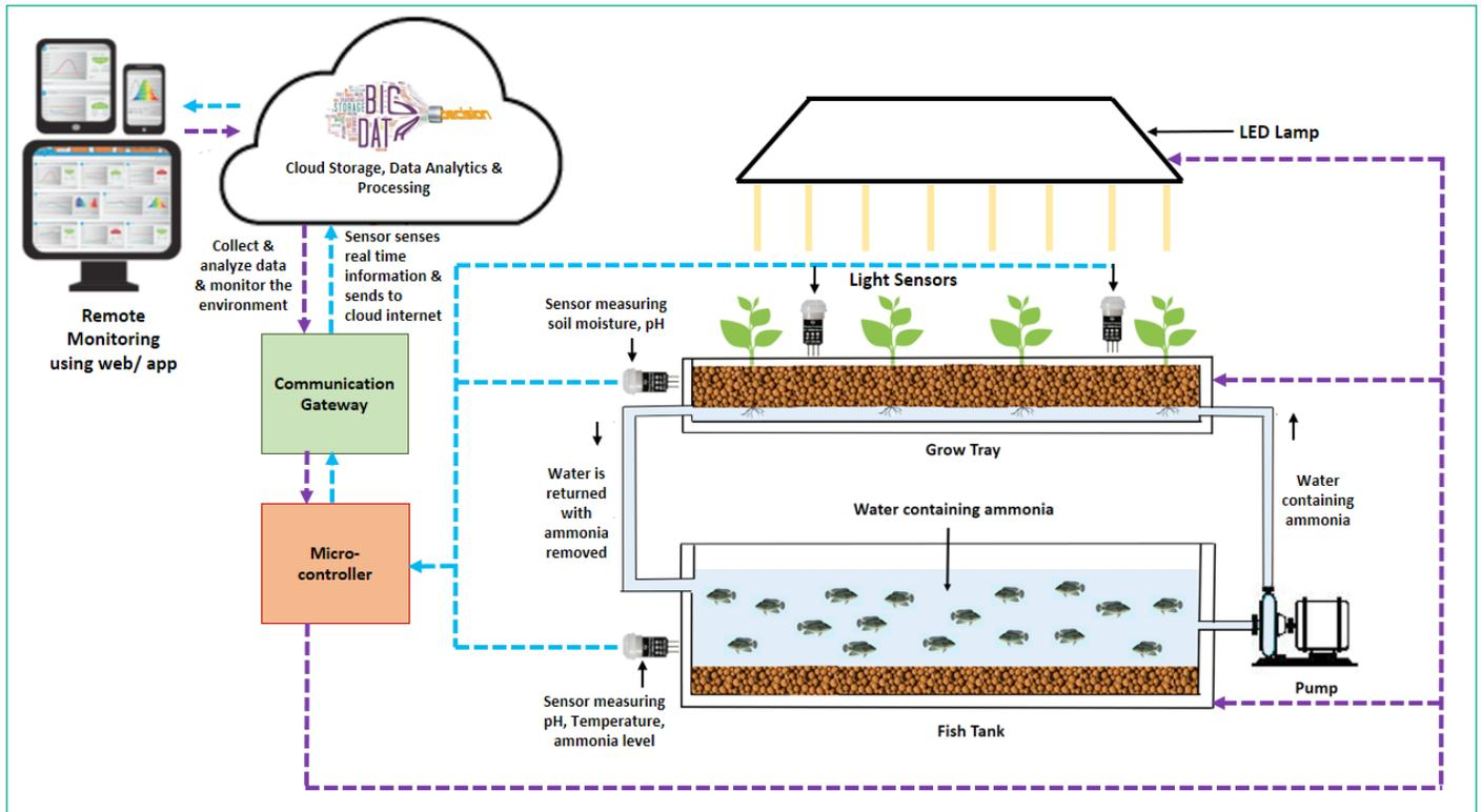
**Figure 4** Schematic Diagram of Implementation of IoT in Vertical Farming
