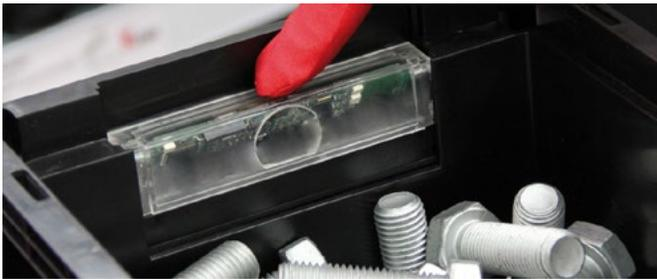
iBin system installed in a bin
