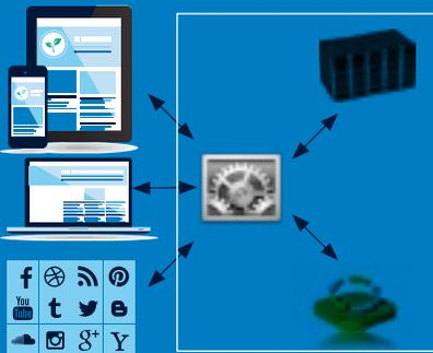
**Cloud-based API manager:** This is used when it is more cost effective to have the gateway external to the enterprise. In this case an enterprise data center is only one of the many service components in the ecosystem.
