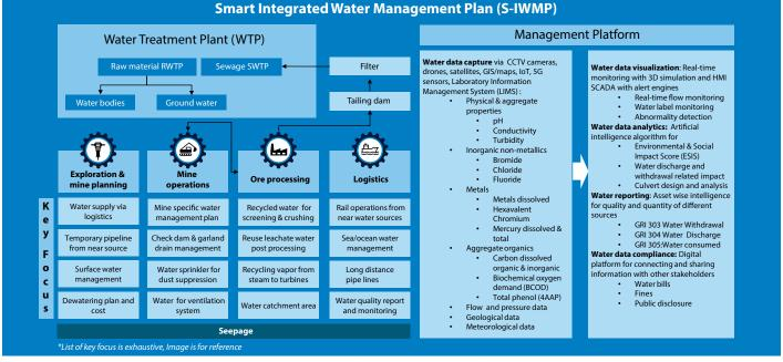
Figure 7: Smart Integrated Water Management Plan S-IWMP
