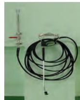
**Centralized high-pressure-water cleaning system** to wash distribution vessels and floors; saves water by 40%
