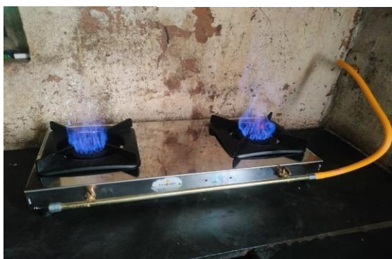
Figure 104: Biogas double-burner stove connected through the H 2 S filter
