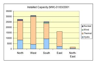
installed power capacity, region wise and source wise, is given in the diagram.
