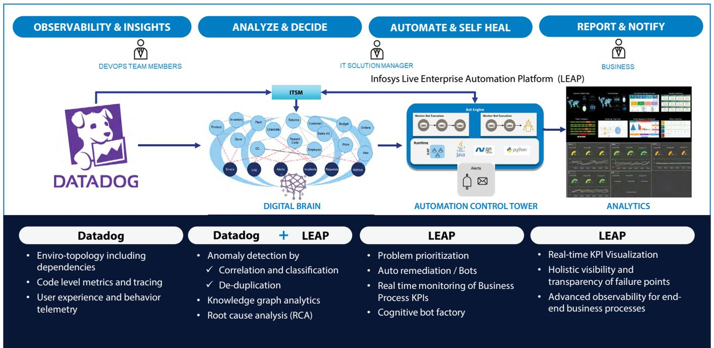
Infosys Live Enterprise Automation Platform (LEAP) ingests telemetry from Datadog into its Digital Brain, which processes it to proactively identify anomalies using AI-led analytics and displays the impact of the anomaly on other aspects of an enterprise's environment. These insights are then fed into a cognitive automation studio for auto-remediation, so that applications can be self-healing and respond to disruptions automatically.
