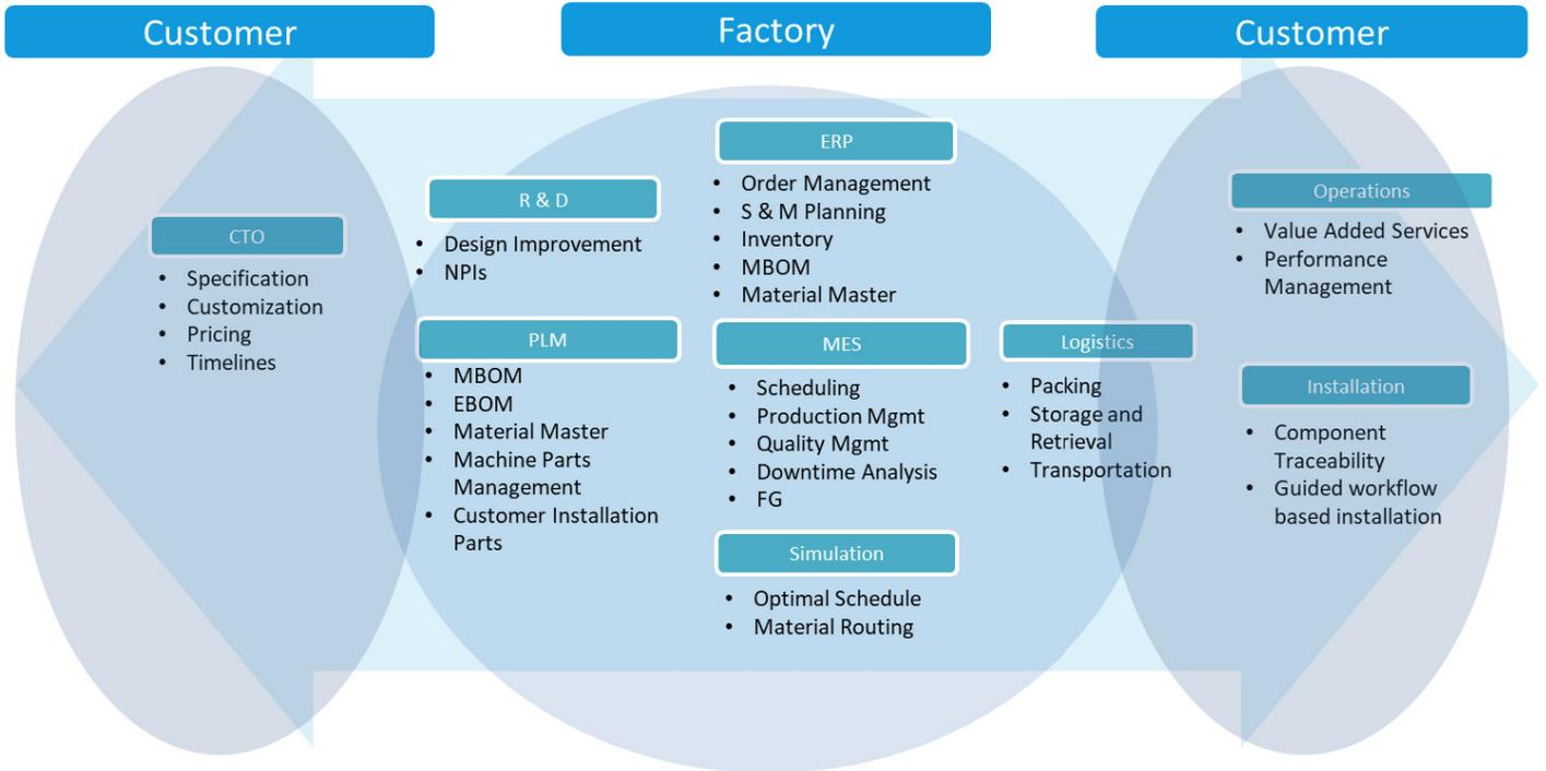
Figure 5. End-to-End digital thread for smart manufacturing
