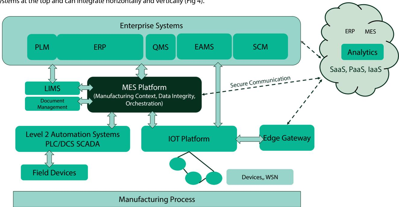
Figure 4. Conceptual view of technical landscape with Core MES for smart manufacturing
