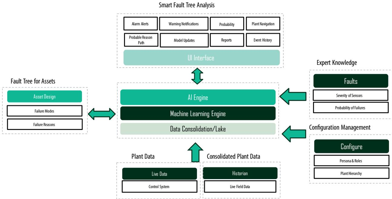
Figure 10: Functional architecture for Smart Fault Tree
