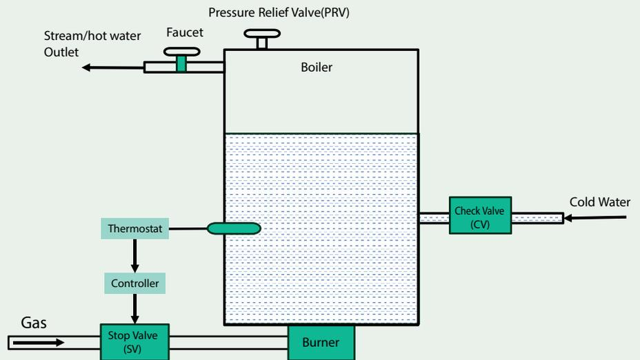
Figure 3: Schematic diagram of the Industrial Boiler and control system
