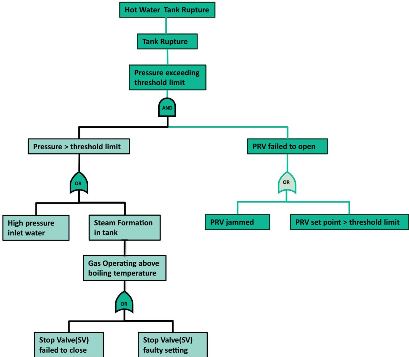
Figure 9: probable failure paths
