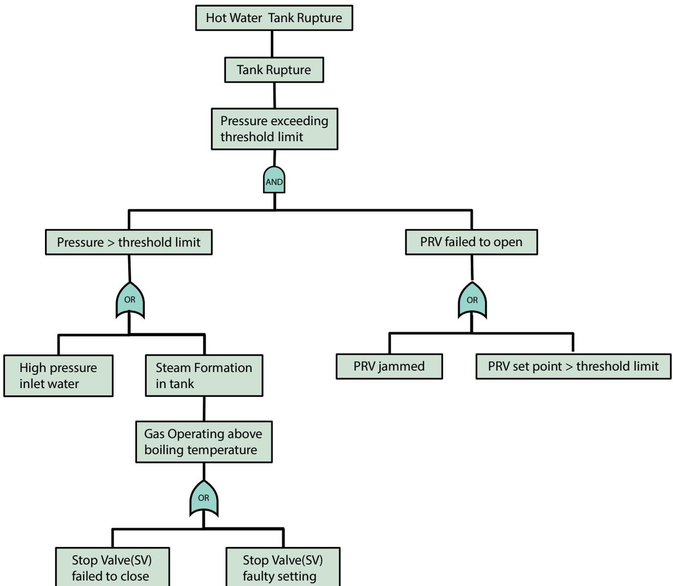
Figure 4: Hot water tank Fault Tree
