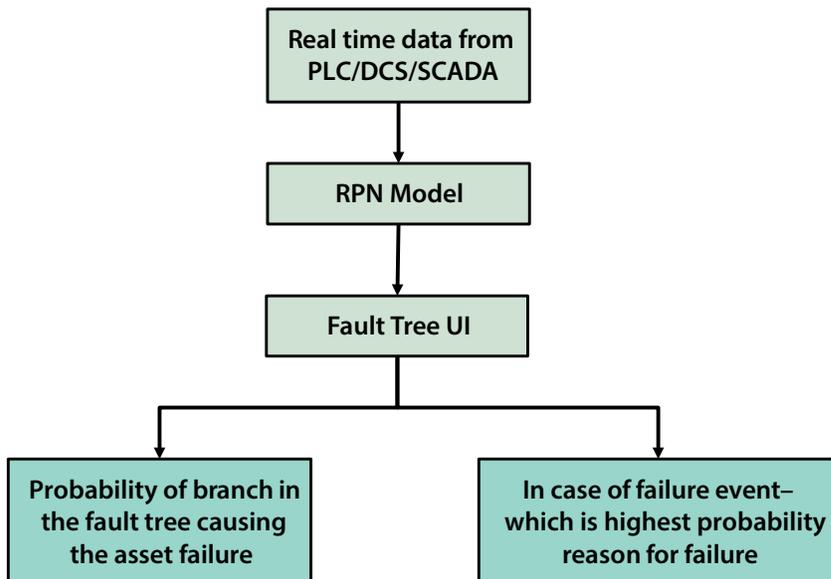
Figure 7: Connecting Smart Fault Tree to Plant live data
