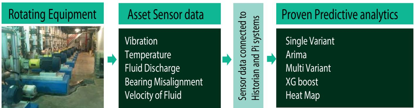
Figure 1: Predictive analytics for Rotating equipment
