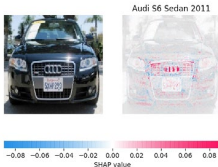
Figure 4: Input image on the left is an Audi car and we see the explanation on the right. The red pixels are contributing more prediction of the class whereas blue pixels are reducing the probability. We see the model is able pick-up the symbolic Audi rings.
