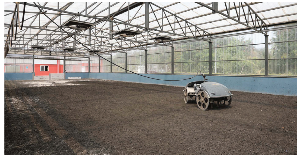
Solar sludge drier in Infosys Hyderabad
