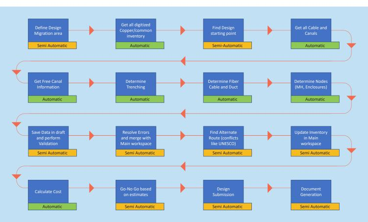
In the below diagram transformation from Copper Network to Fiber Network is depicted: -
