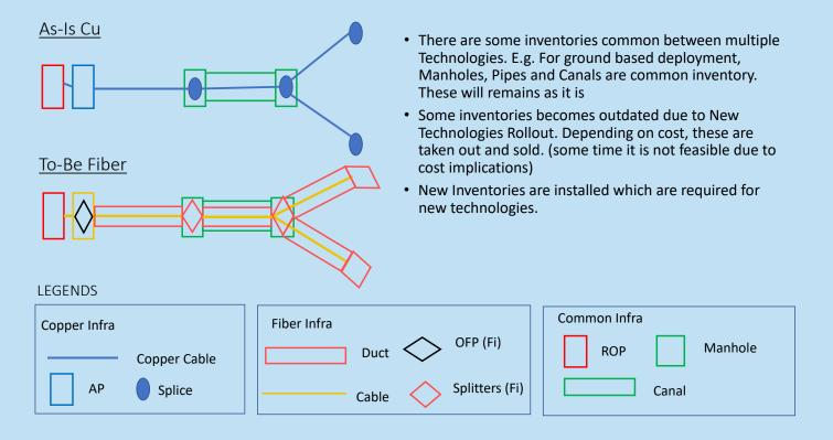
Given below is detailed explanation of copper de-documentation along with fiber rollout:-
